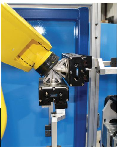
**The complex part designed in Solid Edge and 3D printed with binder jetting technology enables two tools to sit on the end of a robot arm at a 90-degree angle to each other. They must hold a variety of weights for a high-volume precision inspection application.**
