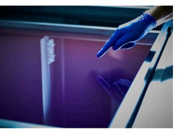
Designed with an open-resin system, offering customers the ability to utilize any commercially available 355 nm hybrid resin chemistry.
